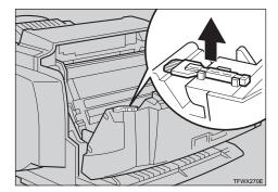
Insert the cleaning brush into the back of the light blue guide until it stops, and then move it left and right four or five times.
